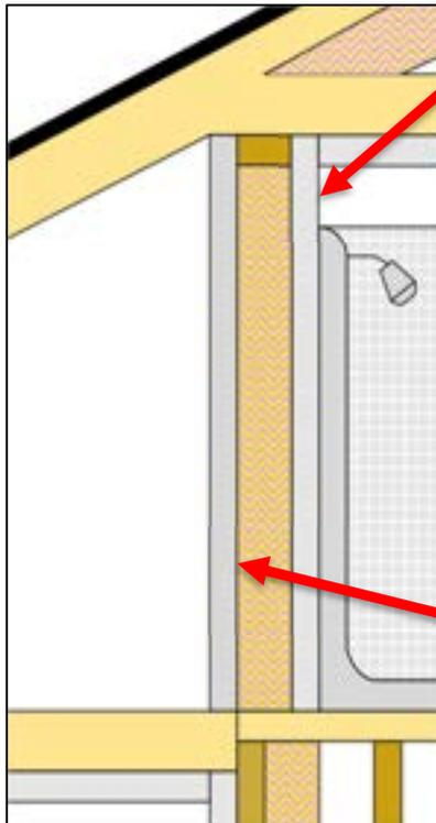
Note that the shower insert has an air barrier installed behind it. This is required by QII.
