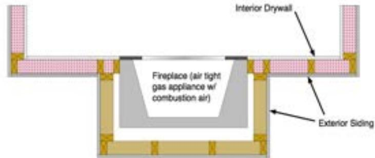
However, this is not acceptable practice to meet QII because it results in an inadequate thermal boundary.
