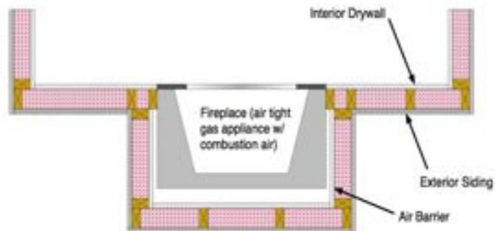
Note that at some point the pop-out will have a top, which must also be insulated. The flue will need to have an air tight flashing around it.
