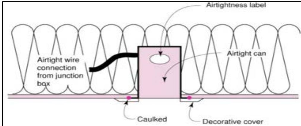
Insulation Contact/ Air Tight (IC/AT) rated can light
