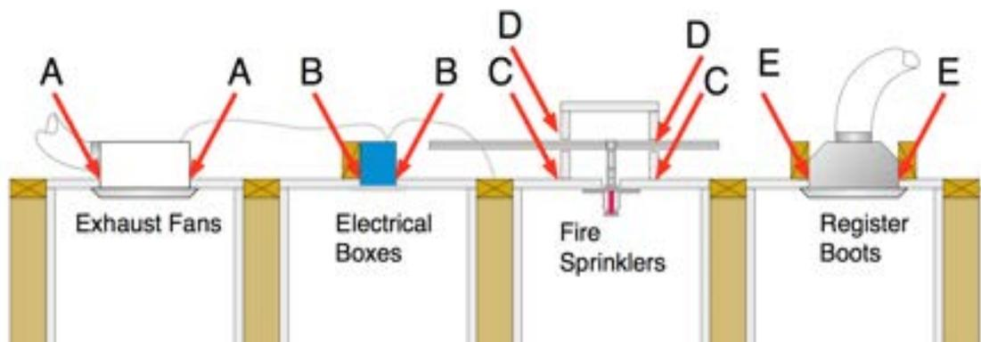
Seal all penetrations to the ceiling drywall when there is unconditioned space above. Best practice is to also do this when there is a floor above.
