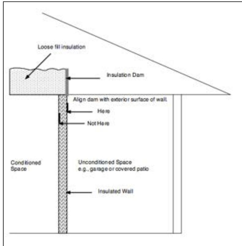
Loose fill extends all the way to the outside of the top plate. In a vented attic where eave baffles are installed, insulation should extend all the way to the baffle.
