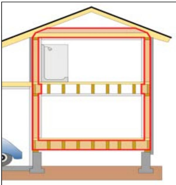
Notice the **air barrier** must be continuous, without any breaks or interruptions where air could readily pass between conditioned and unconditioned spaces. The entire boundary is also properly insulated, except at normal framing members. These should be minimized where possible.
