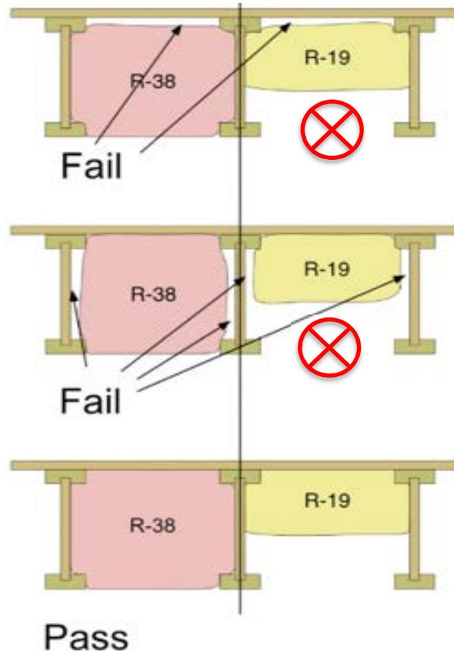
**Note:** "TJI" floor joists pose a particular problem for batt insulation. Make sure that the batts are in contact with the subfloor and are full width batts so that they expand into the side pockets created by the I-beam shape of the joists
