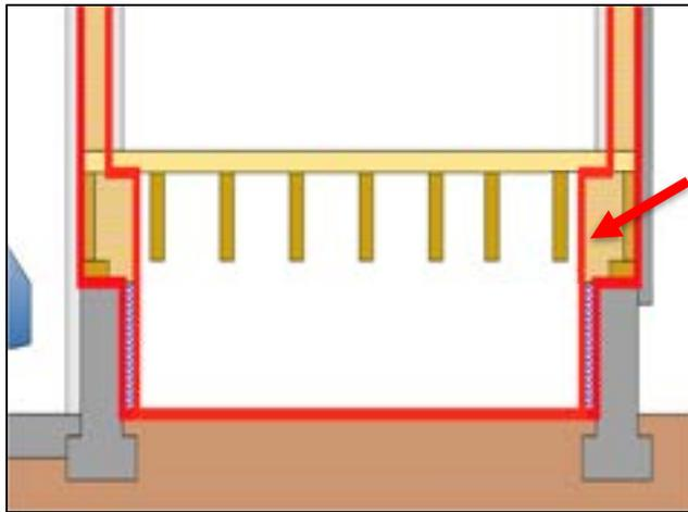
Similarly, if the home had an unvented, conditioned crawlspace, with insulation at the foundation walls, the conditioned boundary would again be substantially different. Conditioned crawlspaces also require a plastic vapor barrier over any bare dirt.
