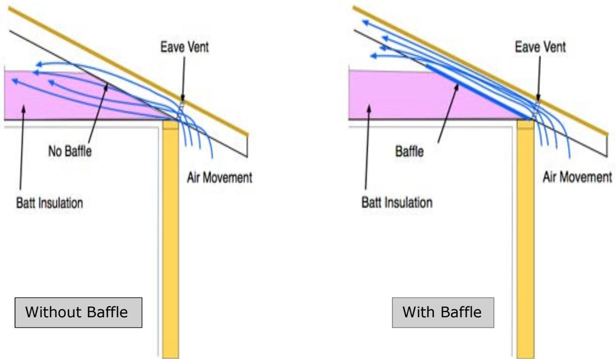
**Note:** Baffles which maintain the net free area are required at all eave vents to prevent air movement under or into the adjacent insulation. Additionally, insulation must be installed to the outside edge of the exterior top plate. Raters shall verify that the baffles maintain the net free area. The open area created by the baffle should be roughly equivalent to the area of the eave vent.
