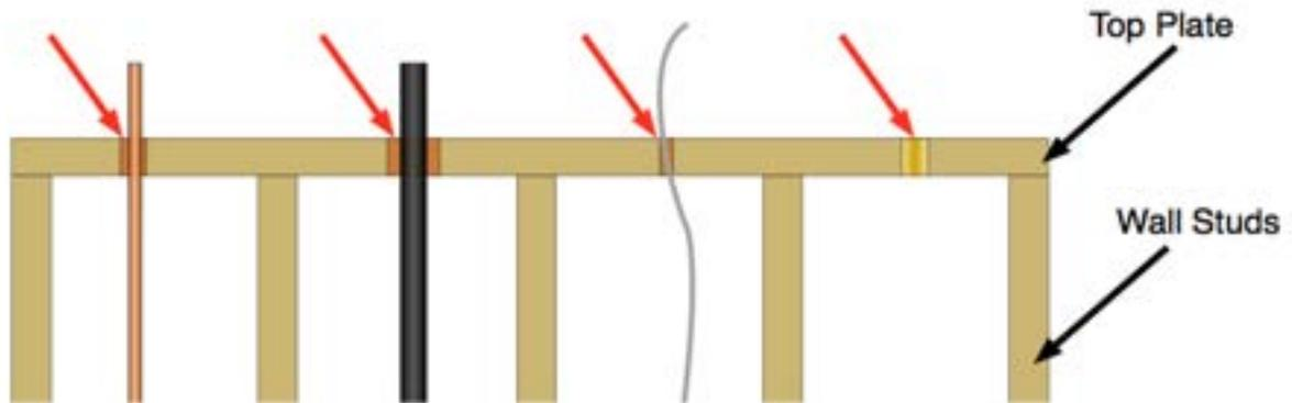
QII protocols require that the HERS Rater verifies that each ceiling penetration is gasketed, caulked, foamed, taped or otherwise sealed as applicable. The following are typical ceiling penetrations that must be sealed and HERS verified.
