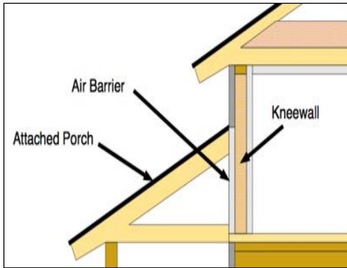
An exterior wall air barrier is required at the intersection of the porch and exterior wall when there is conditioned space on the other side. The exterior wall includes an air barrier where the attic attaches to the conditioned space.
