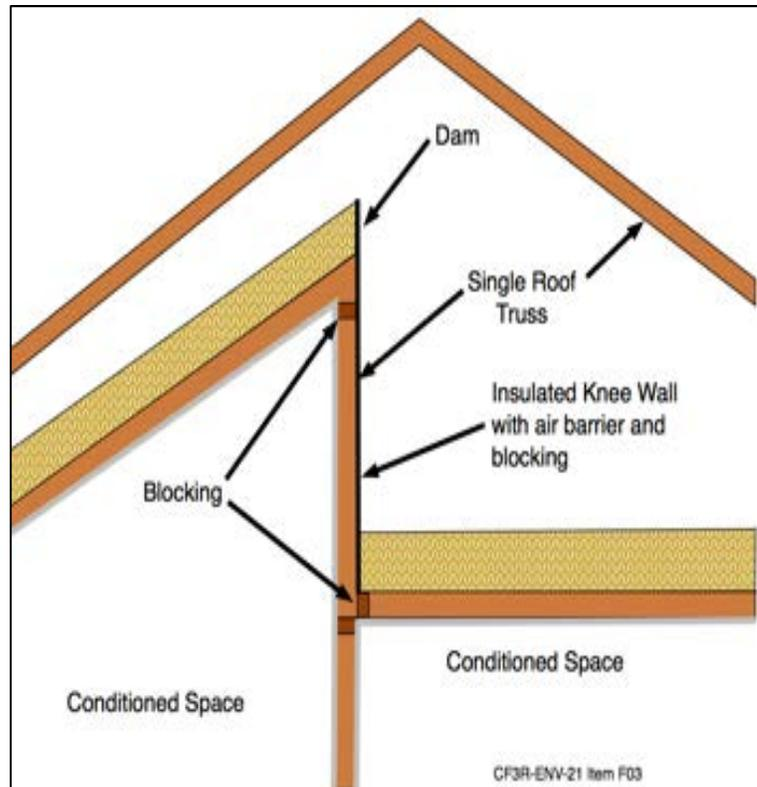
Where a knee wall sits on a subfloor, the spaces between the floor joists must be blocked and sealed to prevent air from moving between the attic and floor joist bays.
