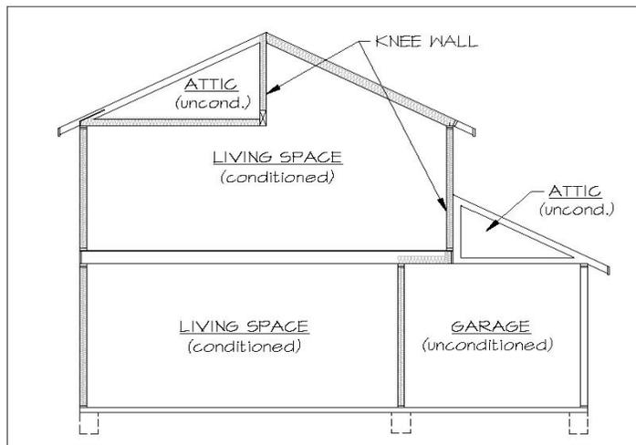
A knee wall is any vertical wall that separates conditioned space from an unconditioned attic
