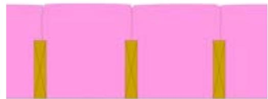
**Note:** *It has been determined that it is virtually impossible to meet the QII requirements with **batts** in an attic ceiling with common roof **trusses** due to the gaps caused by the vertical truss cords.*
