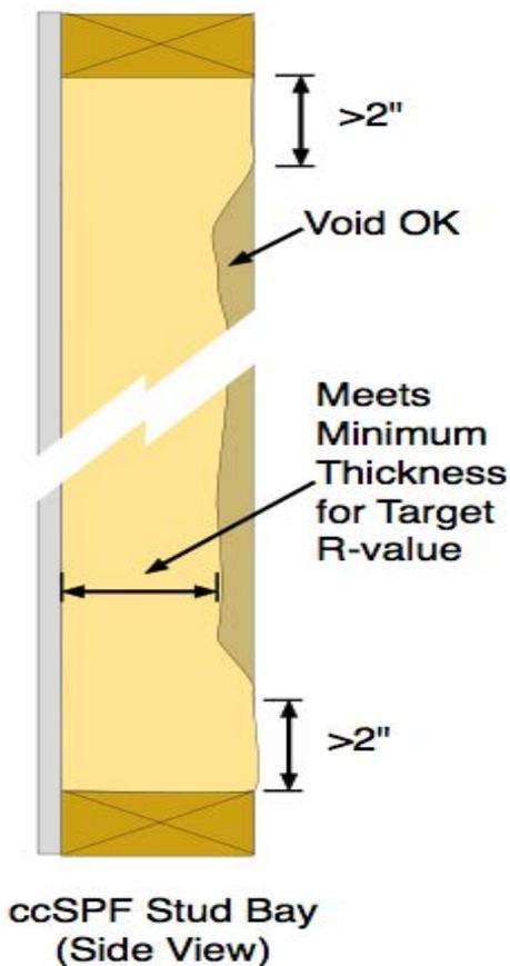
**R-value:** The total R-value shall be calculated based on the nominal required thickness of the insulation multiplied by a thermal resistivity of 5.8 per inch. The R-value of ccSPF insulation shall meet or exceed the installed thickness specified in Table 3.5-1 below.
