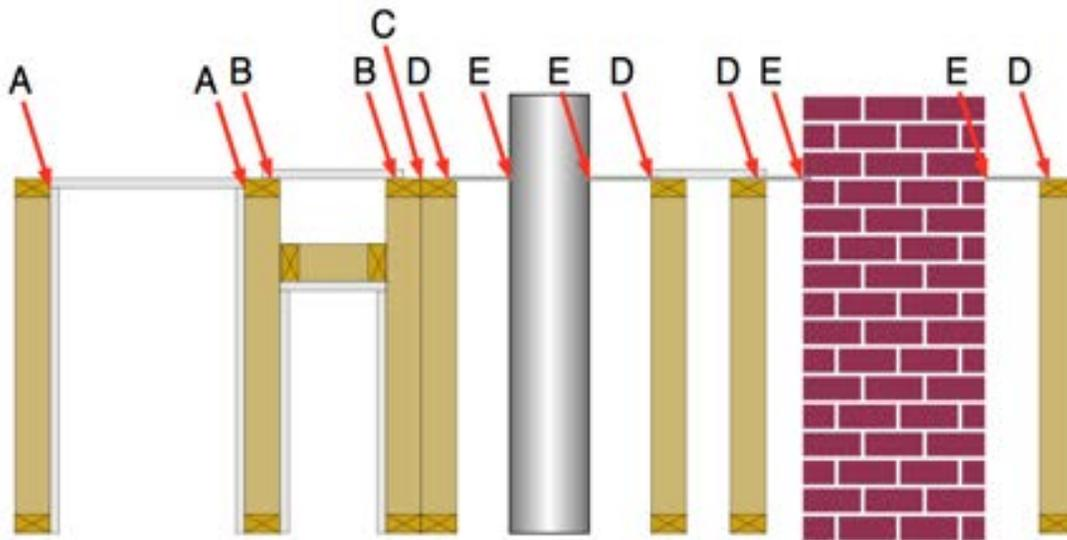
There must be a continuous air barrier at the ceiling level when there is unconditioned space above. Best practice is to also do this when there is a floor above.
