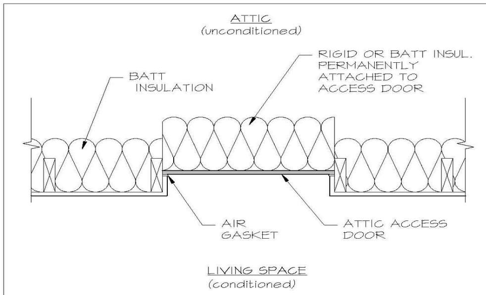
This diagram shows an attic ladder. In this application, weather stripping should be applied to the access door to prevent leakage. The insulation above the access door needs to be insulated to the same R-value as the attic.
